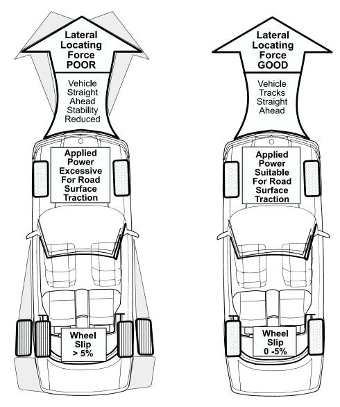
A critical slip ratio of up to 5% between the wheels will cause the traction control regulation to begin. This slip ratio is established when the system detects a wheel spin difference of 2MPH or greater.
