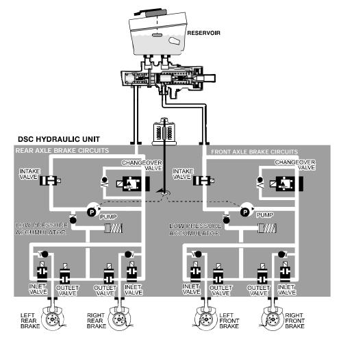
The hydraulic unit consists of an aluminum block containing 12 solenoid valves, 2 pressure accumulators and the return pump.
