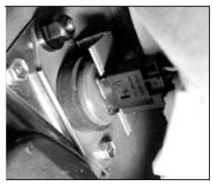
This change of distance between the plates affects the capacitance of the sensor. The evaluation circuitry converts the signal into an analog voltage that is transmitted to the control unit.
