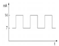
The sensor evaluation circuit is supplied 12V by the MK60 control unit. Output voltage from the sensor is approximately 10V. The control unit counts the high and low current pulses to determine the wheel speed signal.
