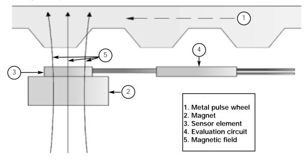
The sensor element is affected by the direction of the magnetic field, not the field strength. The field strength is not important as long as it is above a certain level. This allows the sensor to tolerate variations in the field strength caused by age, temperature or mechanical tolerances.
