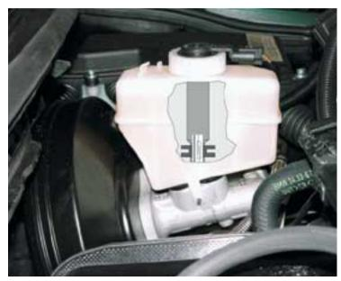
If the fluid level drops below a specified level , the reed contacts open and the MK 60 responds by switching off the ASC/DSC functions.
