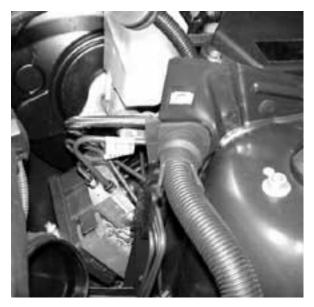
All processing functions for ABS, ASC or DSC are performed by the combined control unit/hydraulic unit. The MK 60 control unit is also responsible for processing the wheel speed signals and providing them to other control units.
