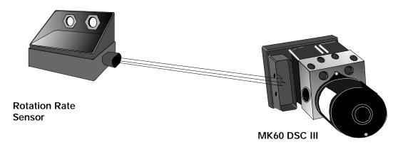
The MK60 DSC III for M.Y. 2002 incorporates a combined Rotation rate and Transverse Acceleration Sensor. The Sensor is connected to the MK60 control unit by the CAN bus. The Z3 version will retain separate sensors until the E36/7 is replaced by the E46/6.
